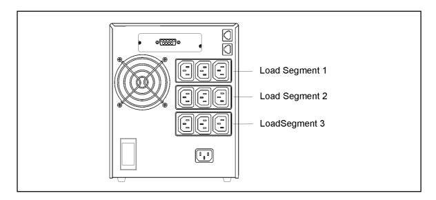
Figure 11. 2200 VA Load Segments
